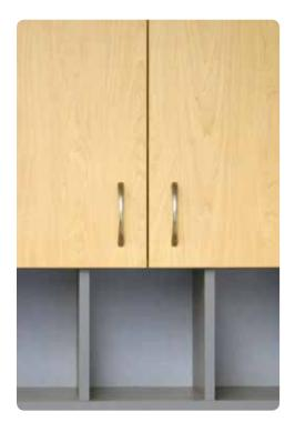
**Standard Top** - Cabinets receive individual modular top constructed of 1-1/4" thick engineered wood with .050" high pressure laminate (HPL) and a phenolic backer sheet. Edges are 3mm PVC on front and .5mm (.020) PVC on sides, bottom and back.
