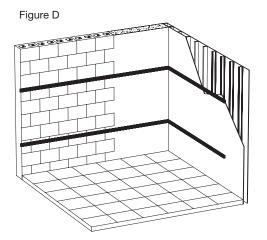
a. Locate the wall substructure along the fastener location chalk lines.
