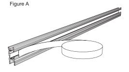
**Step 1** - Unroll fastener concealment vinyl and cut to required length with scissors. See Figure A.
