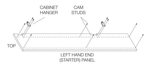
b. Mount cabinet hangers in the pre-drilled mounting holes in the end panels at the locations shown. Note that the mounting screws are located beneath the cabinet hanger when mounted correctly. (Figure O).
