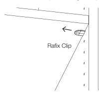
Step 2: Once Rafix Clip is slid into unlocked position, lift shelf up.
