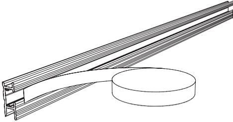
**Step 1** - Unroll fastener concealment vinyl and cut to required length with scissors. See Figure A.
