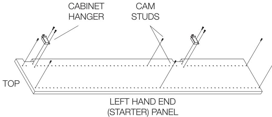
b. Mount cabinet hangers in the pre-drilled mounting holes in the end panels at the locations shown. Note that the mounting screws are located beneath the cabinet hanger when mounted correctly. (Figure O).
