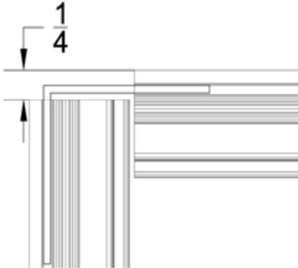
Cut the track, when necessary, to the proper lengths.
