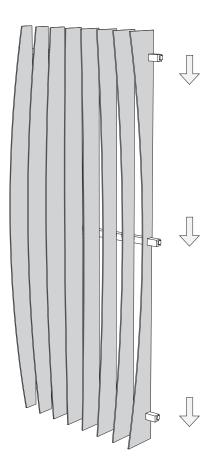
Carefully let the fins down making sure that all of the rail clips engage with the wall clips.
