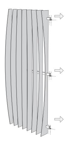
Lift upwards above brackets, and then push backwards until there is contact with the wall.
