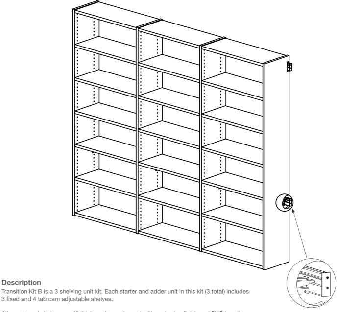
All panels and shelves are 1" thick engineered wood with melamine finish and PVC banding.
