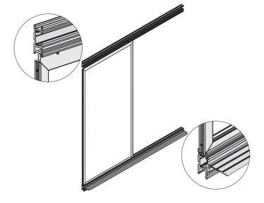
Upper and lower horizontal mounting tracks are required for proper installation of Elements® Tiles. Tiles mount between the upper and lower tracks. They rest on the lower horizontal track and are secured with HTNSS available set screws see **Elements Track Installation Hardware.**
