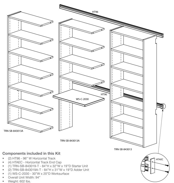
Note: Starter unit widths include the width of the shelf plus the width of two end panels (shelf width plus 2"). Adder unit widths include the length of the shelf plus the width of one intermediate panel (shelf width plus 1"). Overall base cabinet height is expressed including the 6" space between the floor and the bottom of the base cabinet.
