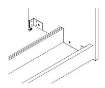
**STEP 1 - Loosely Attach Z Brackets to end panel.** Finger tight only for now.
