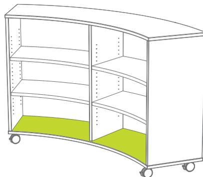
**Step 4:** Select PVC or wood edge for top, ends, intermediate panels and fixed base (shelf) edges.
