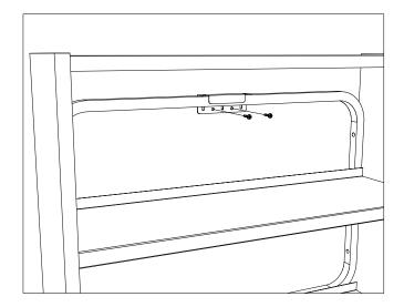
For floor anchoring, fasten to the inside face of the desired shelving end or adder panel at a location below the lower shelf using  $#10 \times 3/4$ " screws. Fasten to the floor with anchors provided by owner/installer.
