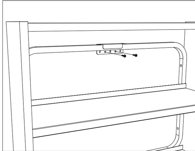
For floor anchoring, fasten to the inside face of the desired shelving end or adder panel at a location below the lower shelf using #10 x 3/4" screws. Fasten to the floor with anchors provided by owner/installer.
