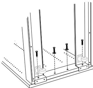
**STEP 2 - Attaching the caster frame and toe unit to the sides for Mobile Bookshelf Unit:**
