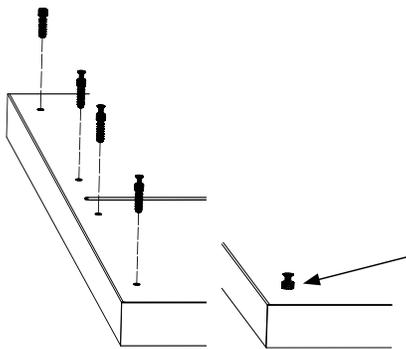
**STEP 1 - Attaching the cams**
