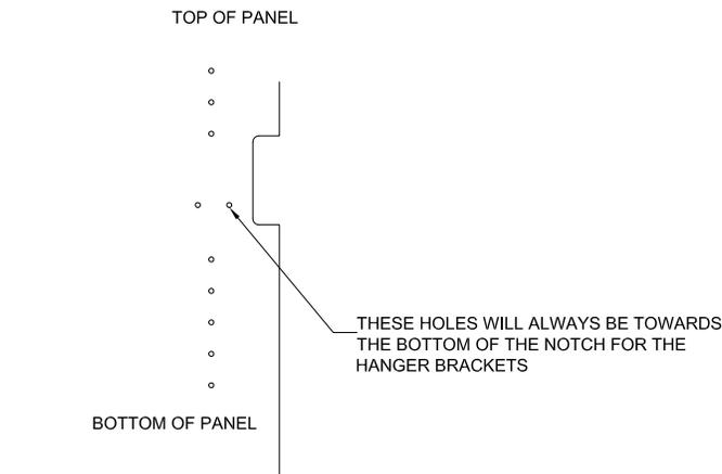
Use Zinc Euro Screw 5mm x 11mm to attach cabinet hangers to the end panel. Inserts are pre-installed 5mm holes in the end panels.
