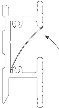
**Step 2** - Slide the bottom edge of the fastener concealment vinyl into the screw channel located in the center of the bottom horizontal mounting track along the entire length of the horizontal mounting track. See Figure B.
