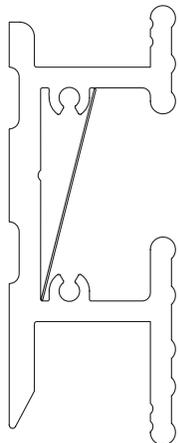
**Step 3** - Gently push the top edge of the fastener concealment vinyl behind the top lip of the horizontal mounting track. See Figure C.
