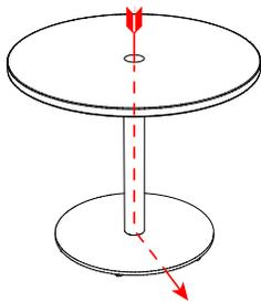
Wire management model has 4" dia column and a step-up place beneath the worksurface. Cable exits beneath the disc base.
