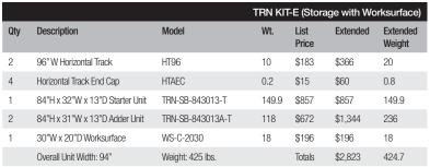
**Note:** Starter Unit widths include the width of the shelf plus the width of two end panels (shelf width plus 2"). Adder Unit widths include the length of the shelf plus the width of one intermediate panel shelf width plus 1"). Overall base cabinet height is expressed including the 6" space between the floor and the bottom of the base cabinet.
